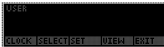
Figure 3 User level soft key group
